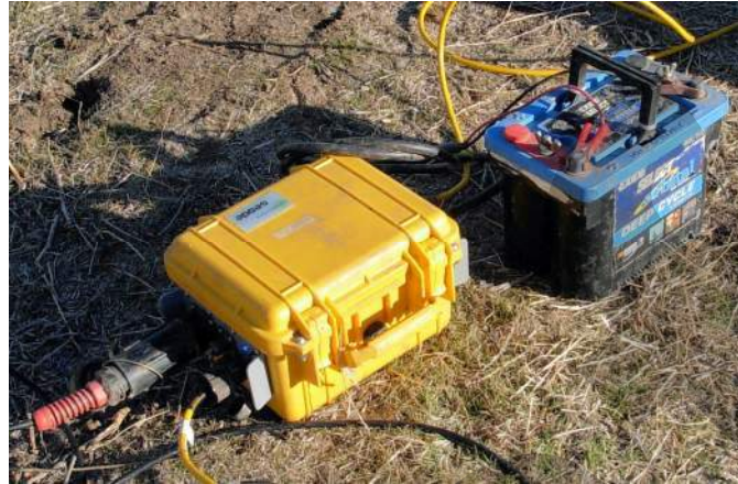
Figure 1: Geometrics Geode 24-channel engineering distributed array seismograph with 12-volt battery power source.
