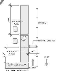
Figure 9.3 Single Lane Screening Station Diagram
