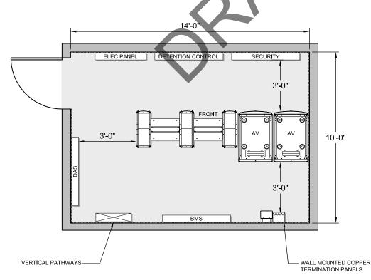
Figure 17.2 Typical Smaller Courthouse MDF Layout
