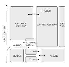
Figure 6.2 Jury Assembly Suite Adjacency Diagram
