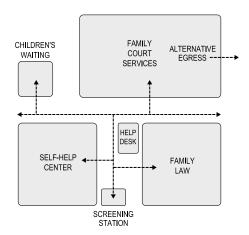
Figure 7.4 Special Services Adjacency Diagram
