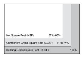
Figure 2.3 Courthouse Efficiency Factors
