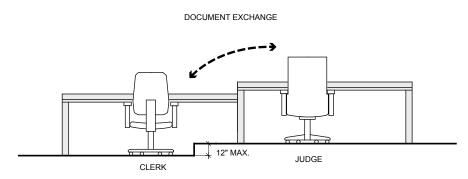
Figure 5.4 Bench and Clerk Elevation
