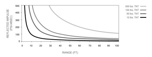
Figure 4.3 Impulse Decay with Distance
