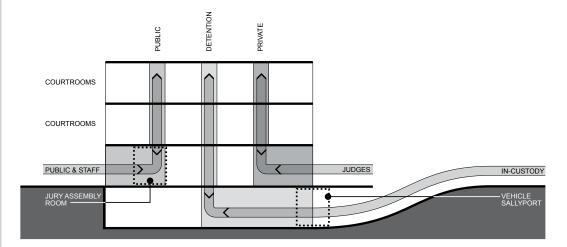
Figure 2.1 Section Showing Three-Part Circulation System
