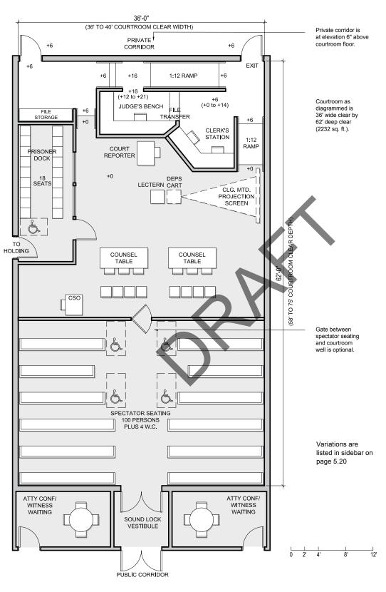
Figure 5.24 Arraignment Courtroom (Central Bench)
