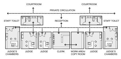
Figure 5.17 Combined Chamber Layout
