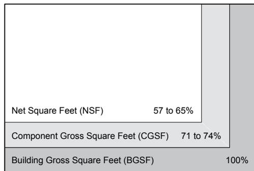
Figure 2.3 Courthouse Efficiency Factors
