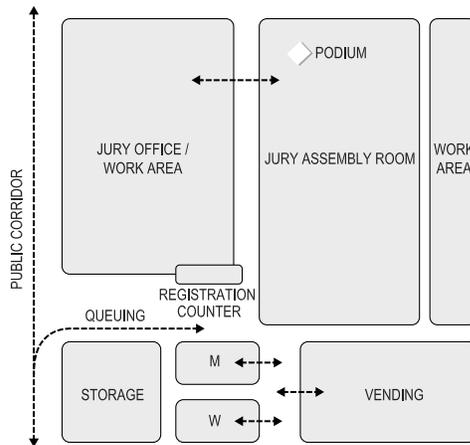
**Figure 6.2** Jury Assembly Suite Adjacency Diagram
