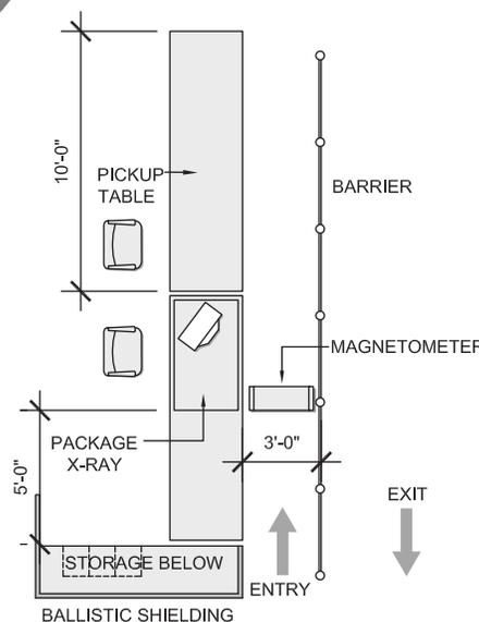
**Figure 9.3** Single Lane Screening Station Diagram
