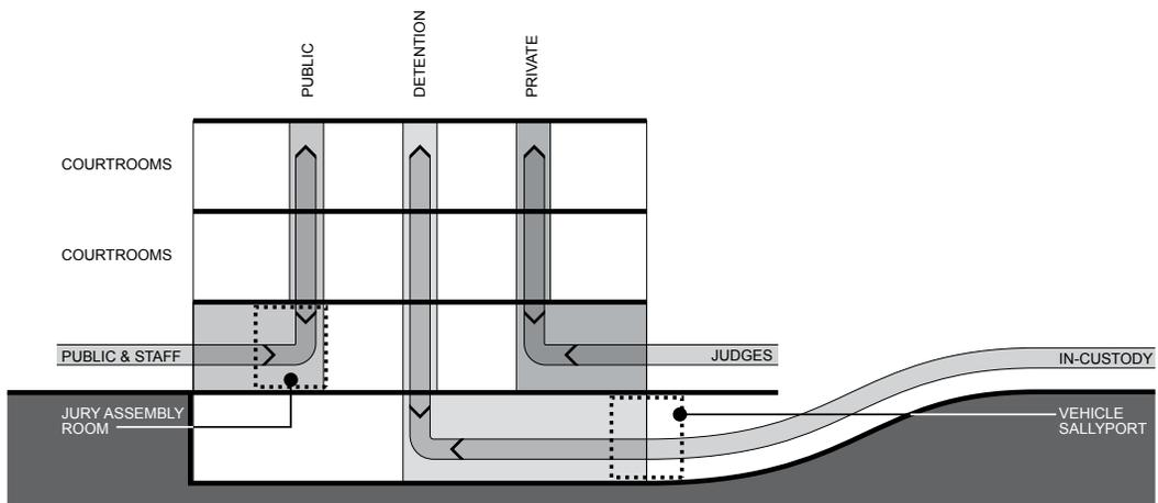
**Figure 2.1** Section Showing Three-Part Circulation System
