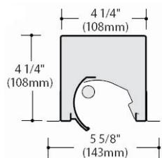
**Figure 16.2** Linear Wallwasher Fixture
