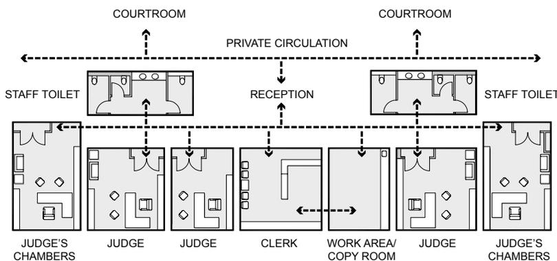
Figure 5.17 Combined Chamber Layout
