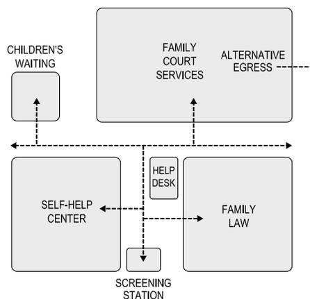
**Figure 7.4** Special Services Adjacency Diagram
