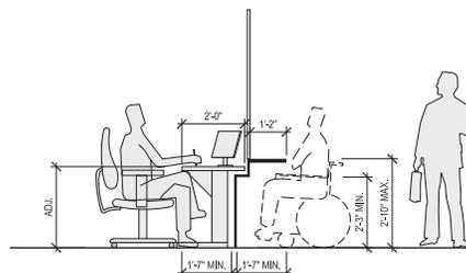
Figure 6.4 Transaction Height Counter
