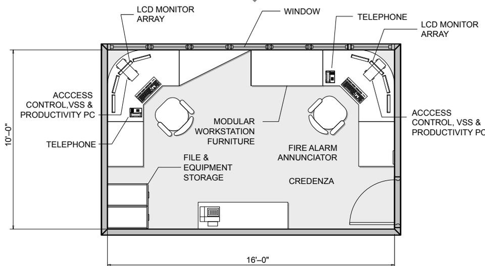
**Figure 4.4** Plan of Security Control Station
