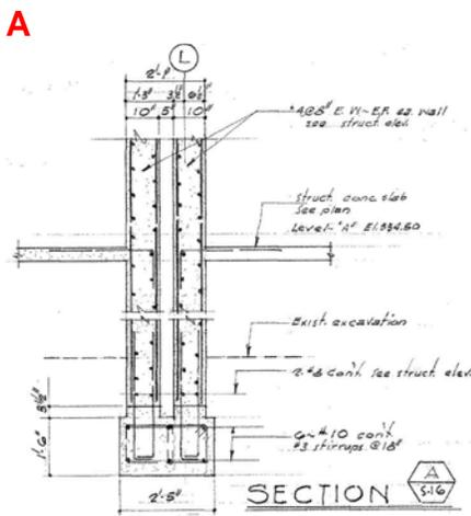
Section at Seismic Joint
