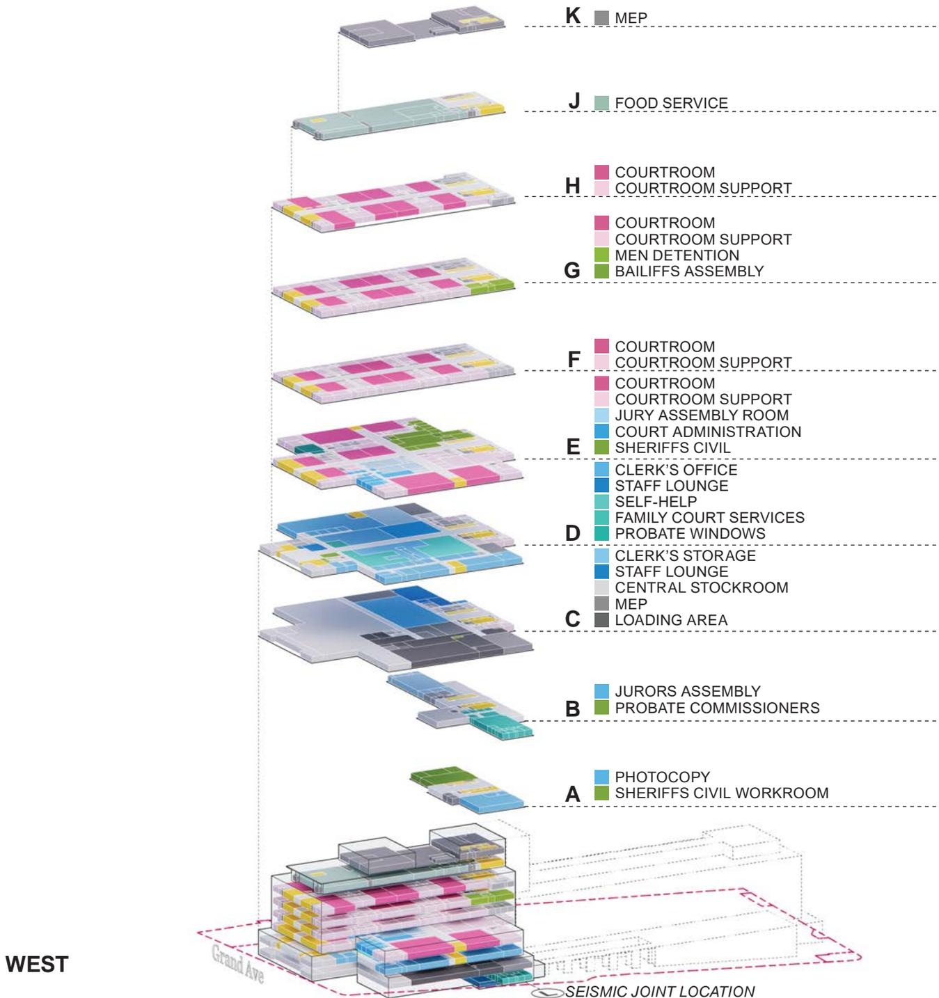
Axonometric diagram of Stanley Mosk Courthouse, levels are separated and color coded based on program\*.
