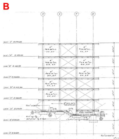
Seismic Concrete Wall Elevation
