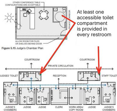
Figure 5.16 Clustered Chamber Layout
