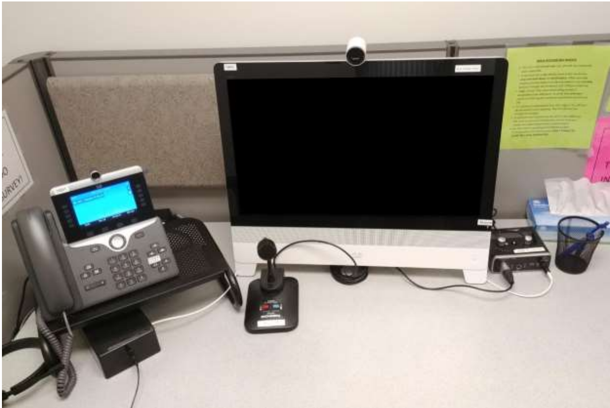
Overview of station. Equipment from left to right: Headset with built in microphone, Cisco video phone, headphone splitter (under the phone), DX80, microphone connected only to the DX80, mixer.
