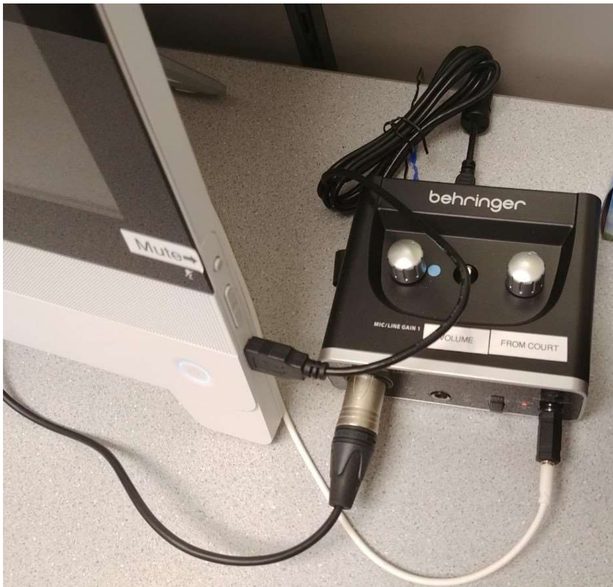
Mixer. Used to connect to a microphone to the DX80 and to allow the headset to hear the sound coming from the DX80.
