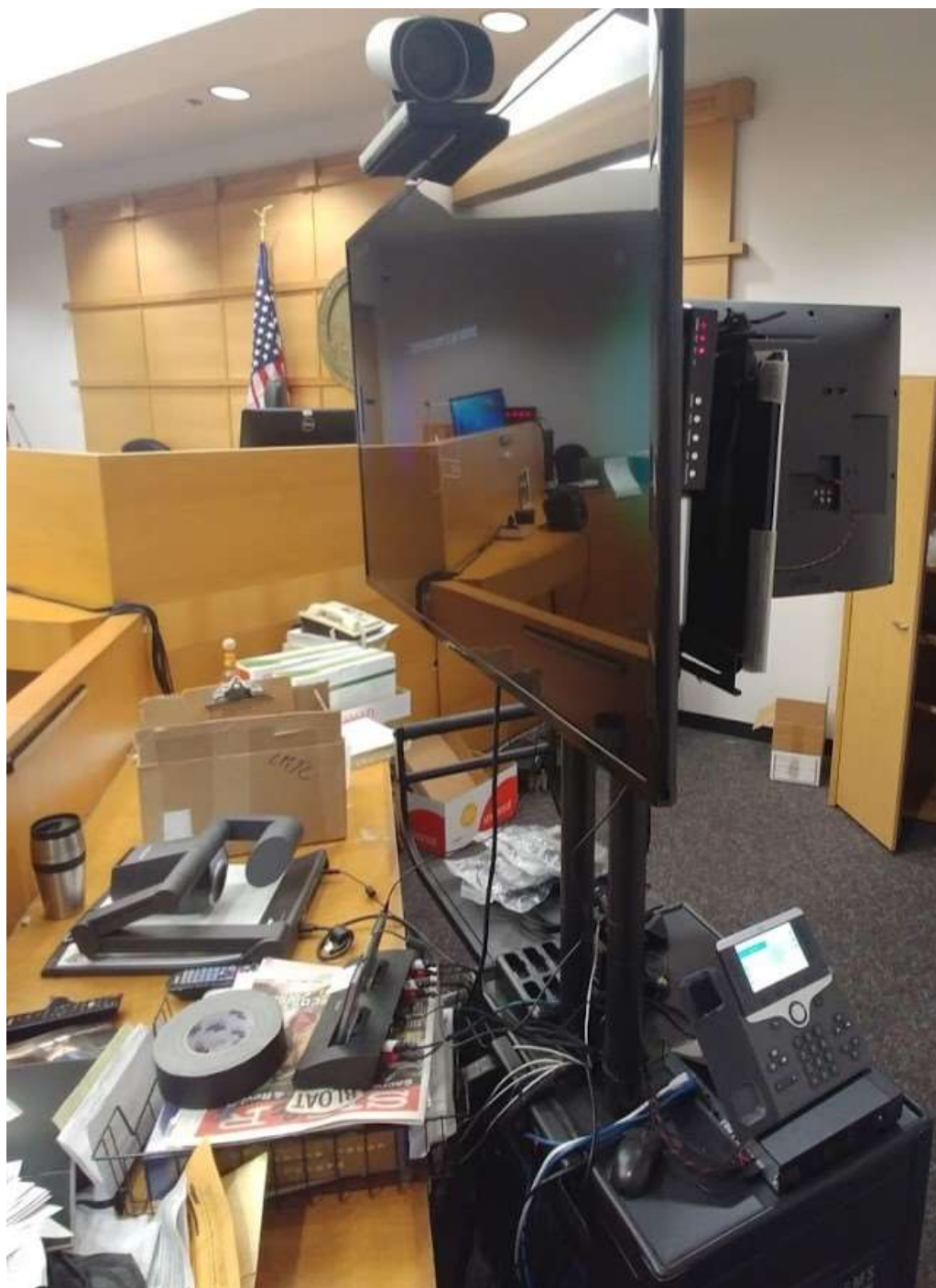
Side view of media cart. Equipment from left to right: document viewer on counter, wireless headsets in charging stations, camera for SX20, courtroom monitor, video converter, SX20, second monitor, and Cisco phone.
