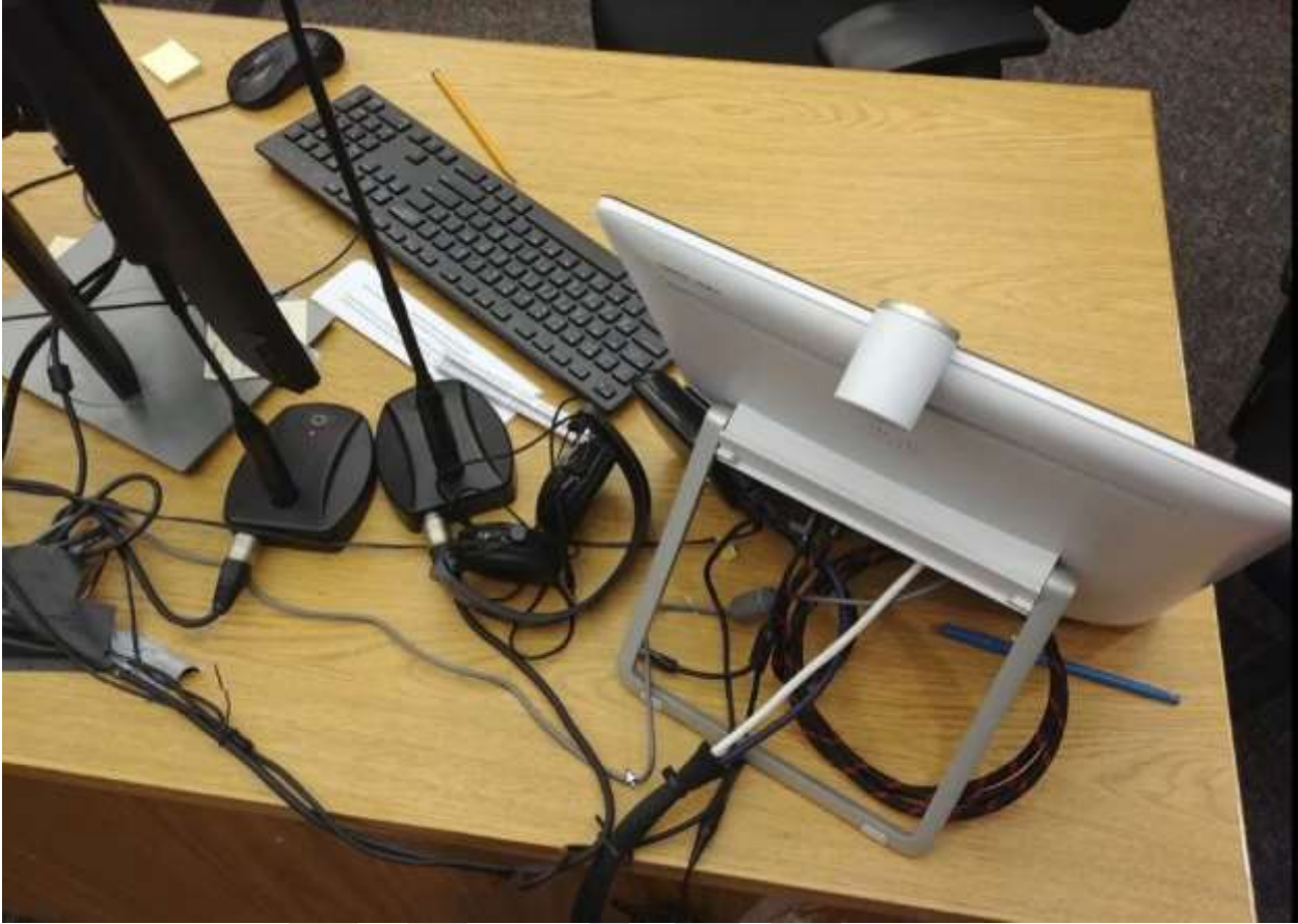
Back of Red Light video station. A rear-mounted mixer is visible to accommodate the speakers and headphones.
