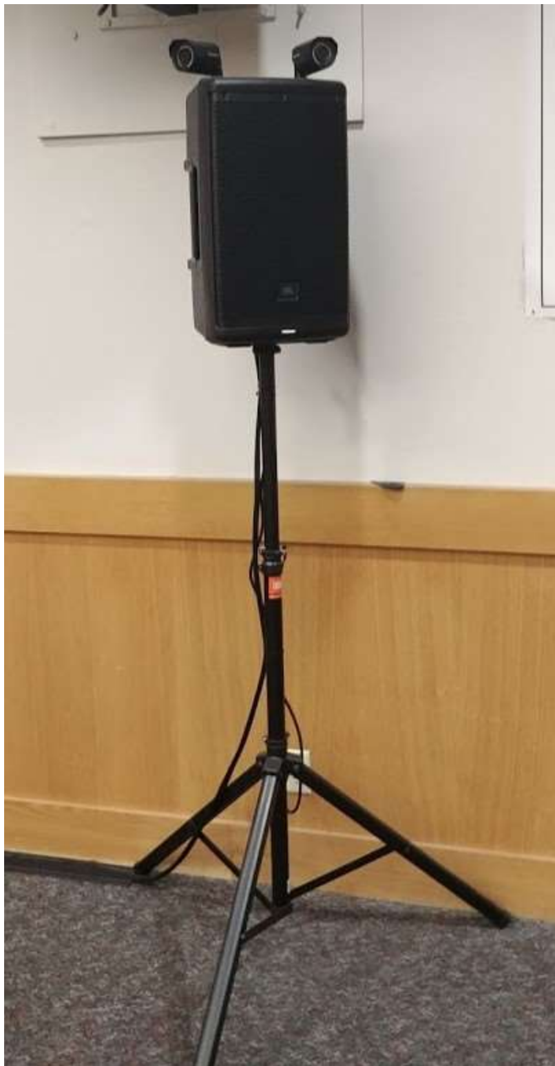
Speaker for projecting sound to courtroom. DX80 would dial into the speaker. Cameras were mounted on top of the speaker for full view of the courtroom. A second speaker was located underneath the bench for the Judge to hear.
