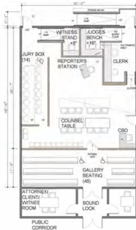
Typical Trial Courtroom Center Bench A (1,850sf; 1,600-2056sf Range) Catalog of Courtroom Layouts for California Trial Courts
