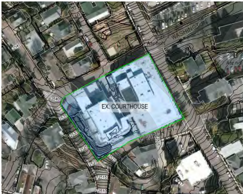
Site Topography for Existing Nevada City Courthouse
