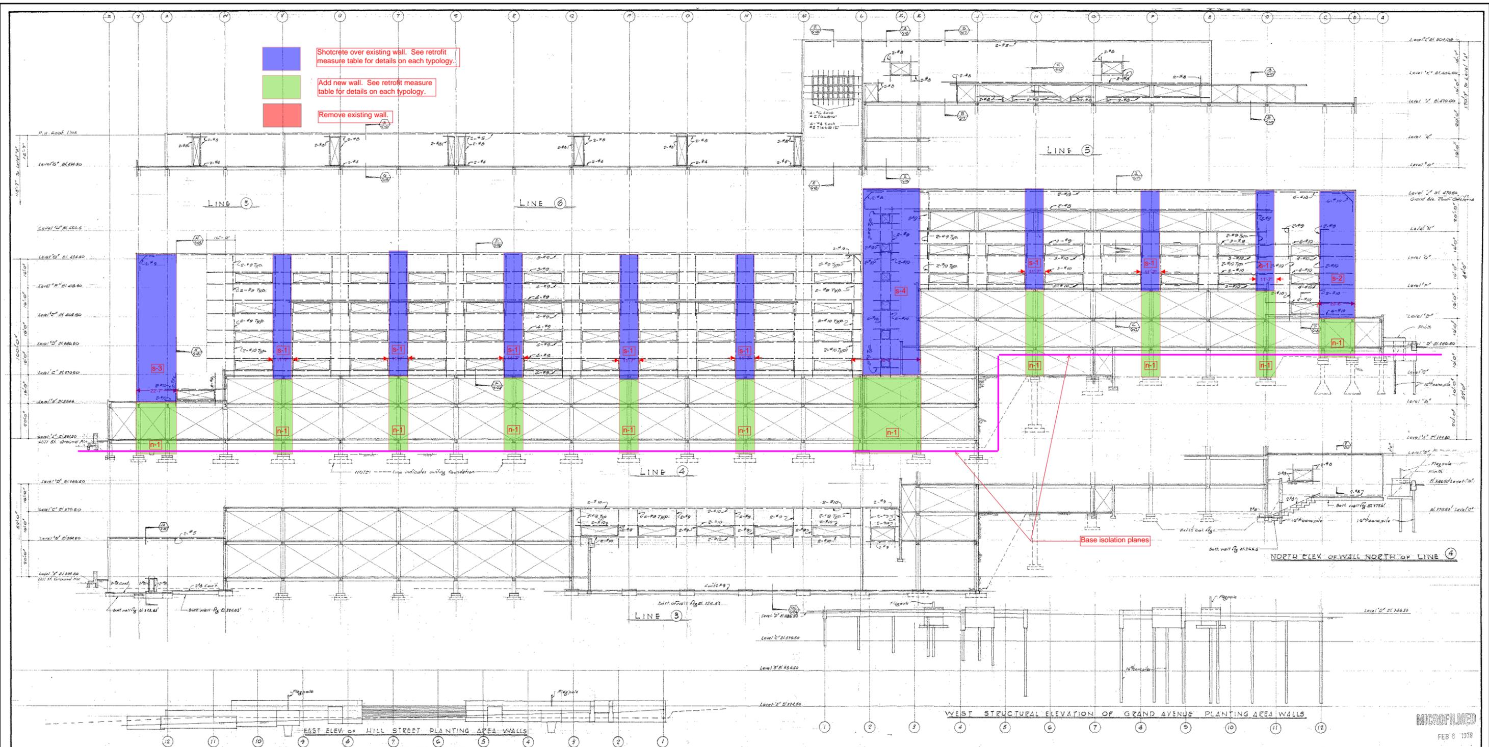
Shotcrete over existing wall. See retrofit measure table for details on each typology.
