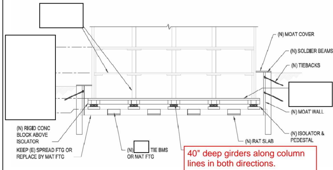
Figure 12.5-15 Typical detail of the isolation system at columns
