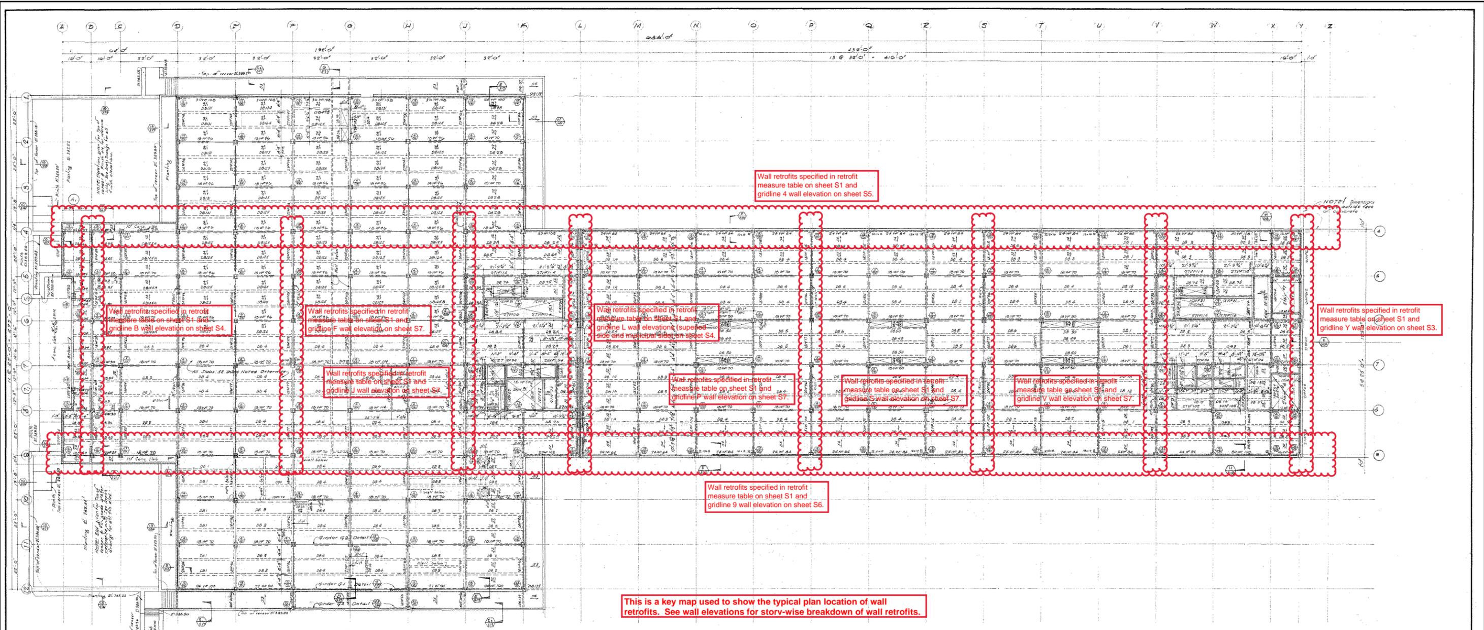
This is a key map used to show the typical plan location of wall retrofits. See wall elevations for story-wise breakdown of wall retrofits.
