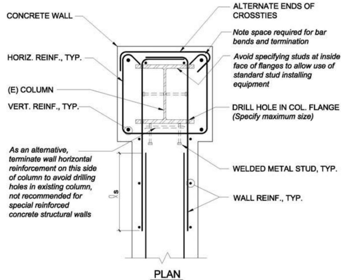
Figure 8.4.2-2: Cast-in-Place Concrete Wall Encasing Existing Column
