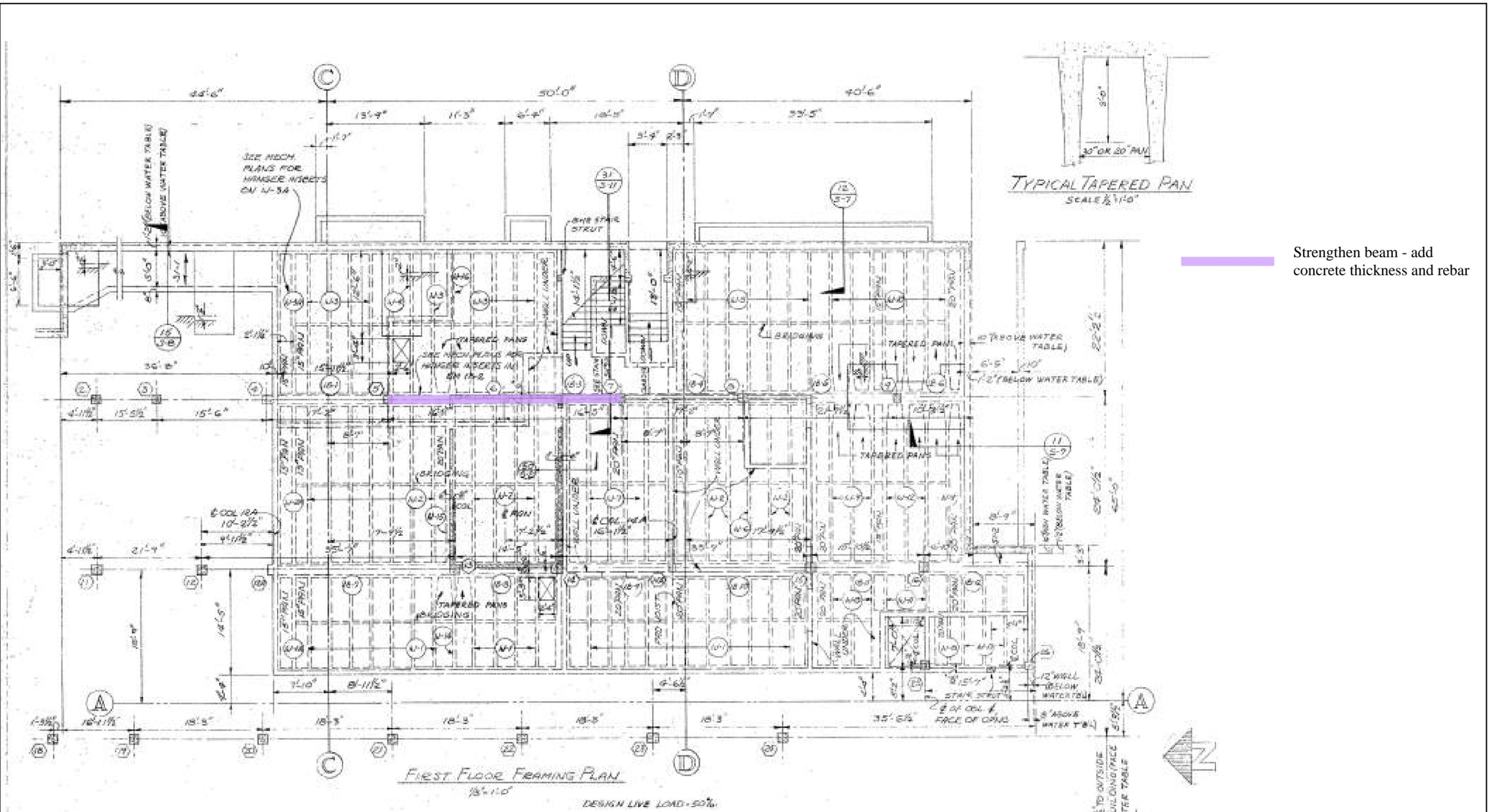
Strengthen beam - add concrete thickness and rebar
