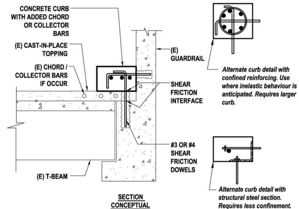
Figure 17.4.1-1: Added or Enhanced Chord or Collector at Floor Perimeter
