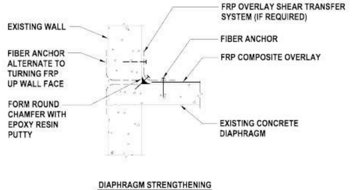
**Figure 22.2.5-1: Shear Strengthening of Concrete Diaphragm Using FRP Composite**
