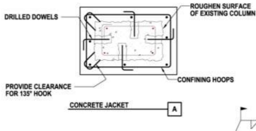
**Figure 12.4.5-1: Concrete and Steel Overlays for Concrete Columns**
