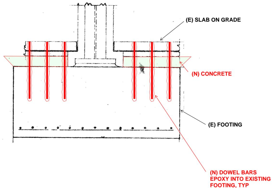
RETROFIT DETAIL 7: Sample Detail of Adding Dowel Bars to Connect Slab on Grade to Footings
