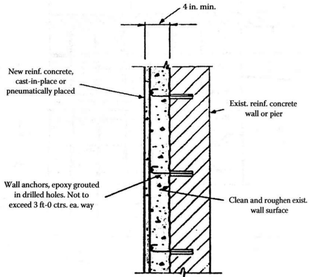
RETROFIT DETAIL 1: Sample detail of Strengthening of Existing Concrete Walls
