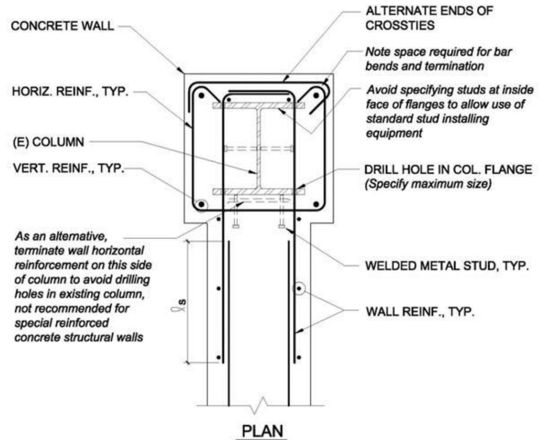
As an alternative, terminate wall horizontal reinforcement on this side of column to avoid drilling holes in existing column, not recommended for special reinforced concrete structural walls
