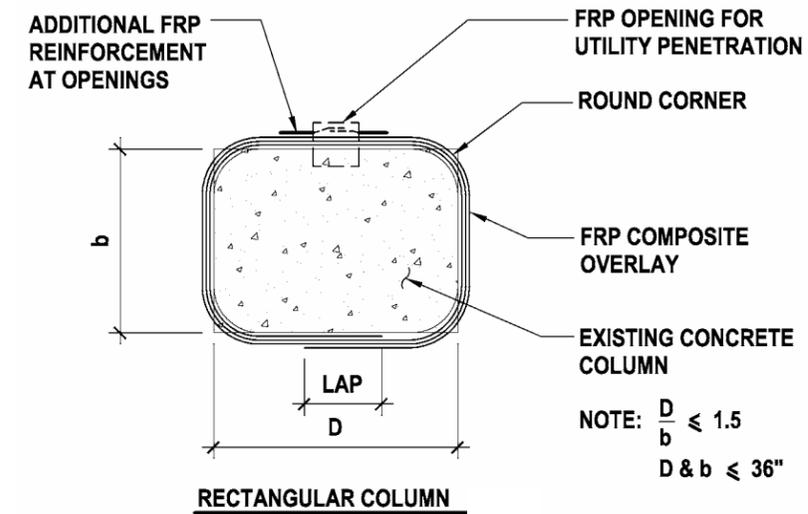
RETROFIT DETAIL 10: Sample Detail of Seismic Retrofit of columns Using FRP Composites - Plan
