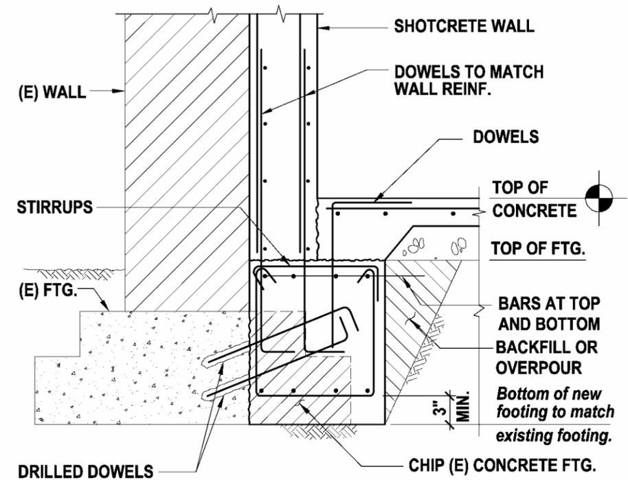
RETROFIT DETAIL 6: Sample Detail of Strengthening Existing Concrete Wall Footing
