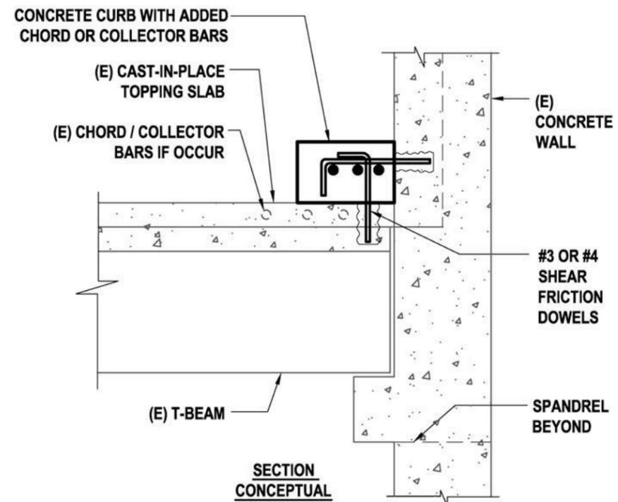
RETROFIT DETAIL 8: Sample Detail of Added Chord to Existing Concrete Wall and Slab Connection
