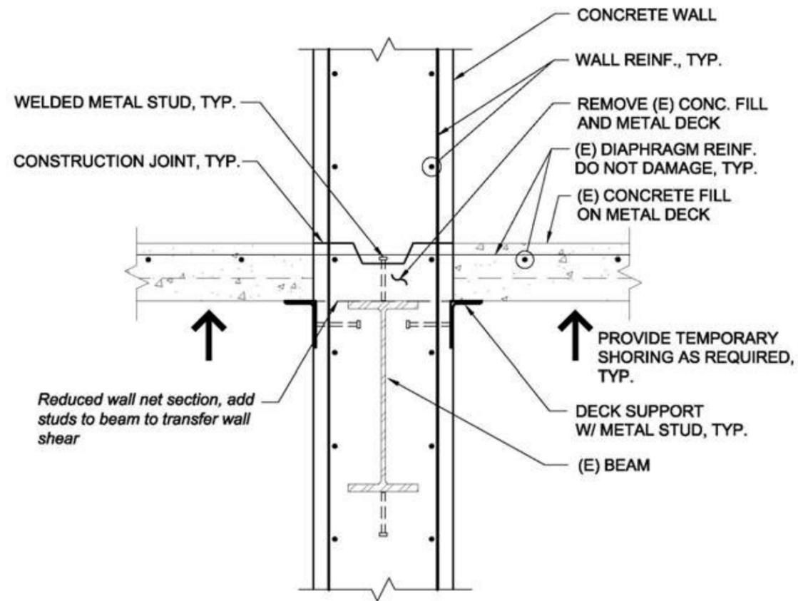
Reduced wall net section, add studs to beam to transfer wall shear
