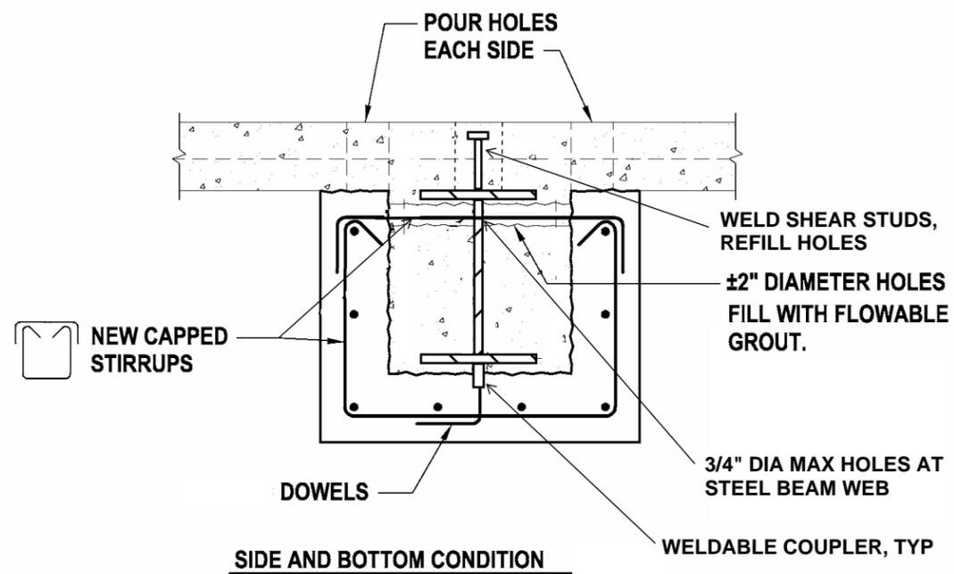
RETROFIT DETAIL 5: Sample Detail of Strengthening of Existing Beam as Collector
