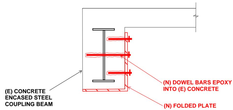
RETROFIT DETAIL 11: Sample Detail of Seismic Retrofit of Existing Concrete Encased Steel Coupling Beams
