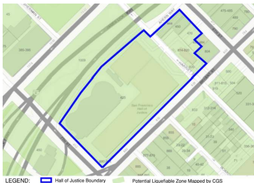
Figure 2: Location of Project Site Relative to Liquefaction Hazard Map For San Francisco
